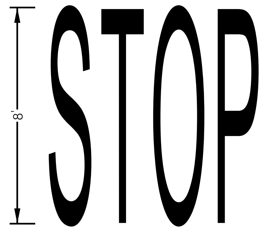
STOP PAVEMENT MARKING DETAIL N.T.S.
