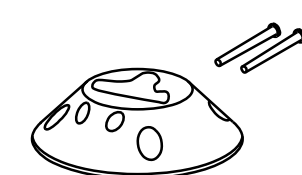
POST IS RETAINED TO BASE WITH 2 PINS
