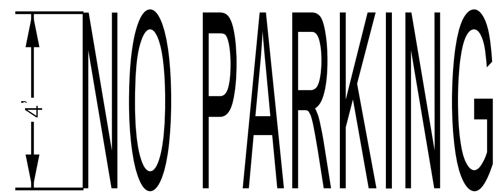
NO PARKING PAVEMENT MARKING DETAIL N.T.S.
